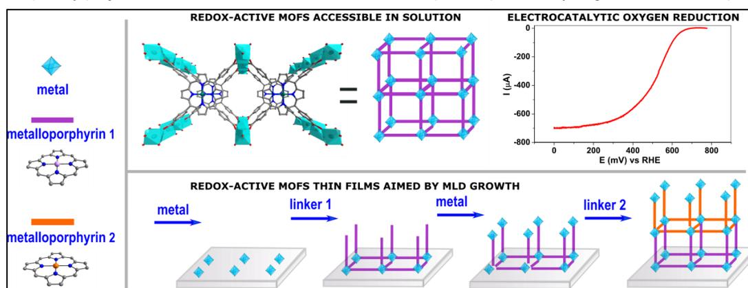
Figure 1: Possible structuration of redox active MOFs by ALD
